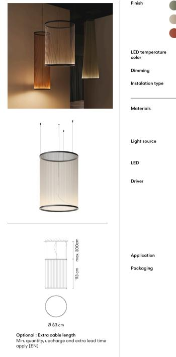
Upper ring: Aluminum Bottom ring: Brass Diffuser: PC- Polycarbonate Threads: PES FR 1 x LED STRIP 50W 48V  $\left| D \right\rangle$ CRI>90 6050 lm 121 2700 K Constant Voltage 90~305 V V 50~60 Hz HZ Dimmable [IP20] [Multi-volt] 50-60Hz 1-10V Hanging lamps 1 Box 0.12 m x 0.93 m x 0.93 m Gross weigth 15.6 Net weigth 10.1 Vol. 0.1037
