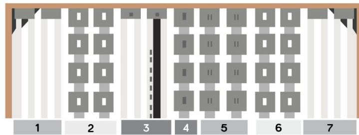
**STANDARD:** Slat system with rectangular frame, rounded edges and epoxy polyester powder coating at 180°C. Slats in beech steam-shaped, inserted in lodgings in the frame 50x25mm. Fixing elements in plastic
