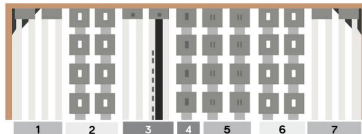
**STANDARD:** Slat system with rectangular frame, rounded edges and epoxy polyester powder coating at 180°C. Slats in beech steam-shaped, inserted in lodgings in the frame 50x25mm. Fixing elements in plastic
